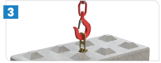
Connect the grab hook to the ring clutch and lift and move the concrete block into the required position.
