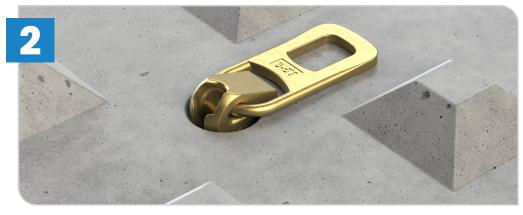
The ring head of the clutch has a locking bolt, which helps safely lock into plate anchors while the concrete panels are in the lifting process.
